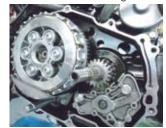
Attach the 0-ring (12mm) to the oil through nut and apply a engine oil to the 0-ring (12mm).
