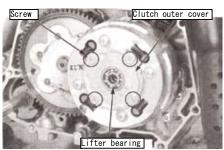
Turn up hooks on the 14mm lock washer. Holding the clutch outer, detach a lock nut with a lock nut wrench.
