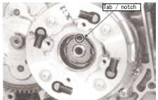
♦ Fix a lifter bearing and gaskets to the supplied clutch outer cover, which please fix onto the clutch outer with four screws.
