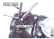
Tighten the bleeder screw to the specified torque.
