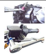
Cut the wiring of the connector (removed from the stock clutch lever) and the wiring of the clutch master cylinder ASSY.
