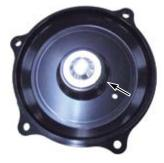
Attach the 0-ring(120mm) to the clutch cover and apply a engine oil to the 0-ring(120mm).
