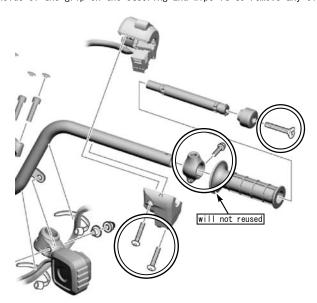
O After the mirror holder is removed, attach the handle switch ASSY. on the Left side. Apply a little Honda genuine adhesive A or Cemedine F540 to the grip rubber, and while the adhesive surface is still dry, rotate the grip and attach the steering handle weight.
