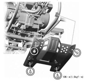
O Remove the two flange bolts 8x16 and four socket bolts 8x16 and 6x12 bolt washers, and carefully remove the under guard pipe.
