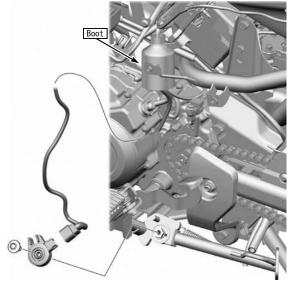
O Remove the four M8x20 flange bolts and 8.5x20 washers and remove the step.
