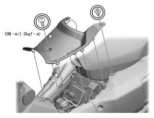
O Remove the 5x14 pan screw and trim clip and remove air cleaner garnish. (note:care about clips)
