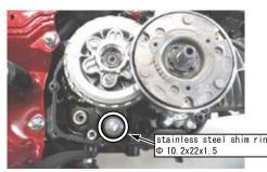
O After removing the oil screen filter and cleaning it thoroughly, assemble the tapered side of the oil screen filter to the crankcase.
