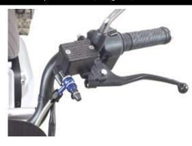
O As shown photo, pre-fix the brake hose fitting to the slim line banjo (straight) and route the hose note:not interfere any part of the exhaust pipe and steering wheel operation.
