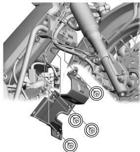
O Remove the four 6x10 screws of the under guard.
