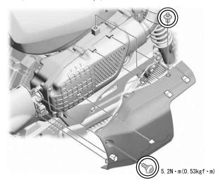
O Remove the 6x14 pan screws and trim clips and remove center cover. | O Remove the M10 flange nut and M8x16 flange bolt that secures the left pivot plate. Remove the M6x20 flange bolt and remove gear shift pedal.
