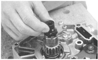
2 . Into a transmission main shaft, put a thrust bearing seat, thrust bearing, thrust washer, and washer in this order, and attach a clutch outer COMP to the transmission main shaft.
