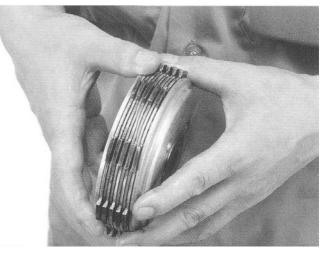
2 Attach the clutch spacer to the transmission main shaft. Fitting the protrusion on the clutch friction disk into the groove in the clutch outer, and also fitting, at the same time, the spline on the clutch center into the spline on the main shaft, attach the clutch assembly.
