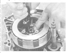
4 . Place four clutch springs into the pressureplate boss, and fix the clutch lifter plate with a flange hex bolt. And tighten it to the specified torque diagonally in a few steps.
