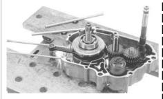
2 . Detach a kick starter spindle, and then a transmission, gear shaft drum and all.
