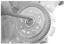
2 . Into a transmission main shaft, put a thrust bearing seat, thrust bearing, thrust washer, and washer in this order, and attach a clutch outer COMP to the transmission main shaft. Set the thrust bearing seat in the location so its protrusion gets stuck on the crankcase, preventing it from rotating
