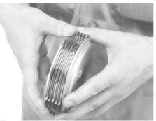
Attach the clutch spacer to the transmission main shaft.
