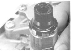
Keep the hooks in close contact with the lock nut.
