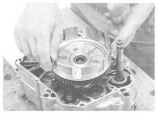
3 Using a gear holder, tighten the lock nut to the specified torque with the crankshaft being seated in detect, and fold back the hook on the lock washer.
