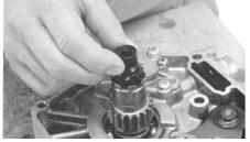
2 . Into a transmission main shaft, put a thrust bearing seat, thrust bearing, thrust washer, and washer in this order, and attach a clutch outer COMP to the transmission main shaft. Set the thrust bearing seat in the location so its protrusion gets stuck on the crankcase, preventing it from rotating
