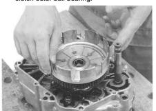
$oxed{3}$  . Using a gear holder, tighten the lock nut to the  $oxed{2}$  . Attach the clutch spacer to the transmission specified torque with the crankshaft being seated in detect, and fold back the hook on the lock washer.
