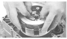
. Fit the supplied external circlip to the groove in the main shaft with the circlip's round corner on the downside.
