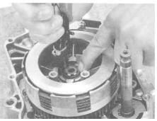
Place four clutch springs into the pressureplate boss, and fix the clutch lifter plate with a flange hex bolt. And tighten it to the specified torque diagonally in a few steps.
