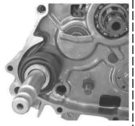
ORemove a return spring and shift-arm spring from O Attach the supplied shift-drum stopper spring the standard gear-shift spindle, and install them to a provided shift spindle.
