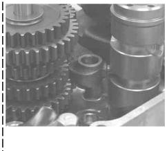
O Attach a provided shift fork "L" on the downside of the countershaft, and the standard shift fork "R" on the top side with the mark facing upward, and install shift fork onto the groove on the shift drum.
