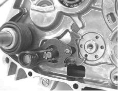
ORemove four shift drum pins from the standard shift drum. Then install a provided shift drum pin and four standard drum pins to the shift drum. Attach a shift drum stopper plate to the shift drum, and apply screw locking agent to the standard hex bolt and tighten it to the specified torque. (Two of the shift drum pins stand taller than others when fixed. Fix a stopper plate by fitting the holes into these two taller pins.)
