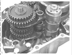
After applying engine oil to the shift-fork shaft, install it to the crankcase.
