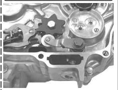
OWhile rotating the mainshaft by hand, rotate the hex bolt, which is fixing the shift stopper plate, in order to check the operation in each gear.
