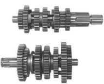
OApply engine oil to a gear and frictional part each on the mainshaft and the countershaft, both of which please fix, as a unit, to the left-side crankcase.
