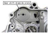
O Fit the shift gear drum stopper plate into the stopper plate setting pin, keeping the marking on the plate visible.
