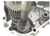
Meshing its friction spring with grooves in the left side
