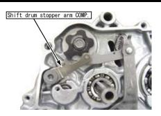
O Turning the mainshaft with hands, turn the knock bolt on the gear shift drum stopper plate with a socket wrench, and check if the gears can shift smoothly.
