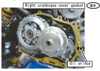
O To attach clamp and right side of crank case cover and tighten to specified torque is divided into several times bolts in diagonal.
