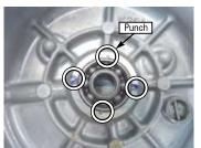
O Clean degreasing gasket surface of right crank case, dowel pins, attach oil orifice, to attach right side crankcase cover gasket new.
