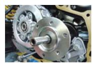
O It fixed primary drive gear and the driven gear or, the oil filter rotor is fixed, washer, a centrifugal filter rotor lock nut mounting and tighten until specified torque. Special tool
