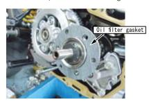
O Clean the oil filter cover in accumulated dirt.
