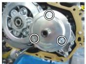
O Right crank case cover and ball bearing of oil filter cover is dropout or confirm the presence or absence of contact mark.
