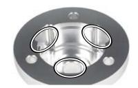
O Use a new oil filter gasket, to attach the oil filter cover. (See previous section)
