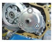
O Oil filter cover, remove the filter gasket.
