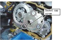
O The oil filter rotor is set, and tighten to the specified torque in the socket cap screw
