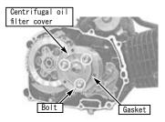
O Primary drive gear and driven gear or, by fixing centrifugal oil filter rotor, and remove centrifugal filter rotor locking nut by special tool.
