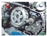
O Attach the included oil filter rotor to the crankshaft.
