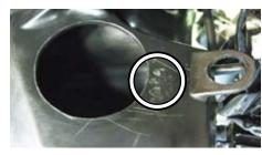
Attach large-diameter air duct. Verify interference of each component, determine position.
