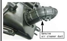
6. Sets the pattern that comes with air cleaner duct mounting holes, to expand processing. Please cleanly remove burrs.
