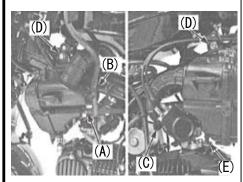
Remove eight screws and remove the air cleaner case cover.
