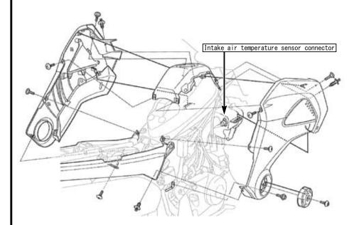
◆ The figure below shows the work contents of GROM (JC61-1300001- JC75-1000001-) and MSX125SF. Same procedure for left and right.
