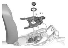
O Remove the 4 screws, remove the air cleaner case cover, and air cleaner element.
