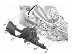
O Referring to the photo, attach ② intake duct to ① air cleaner case cover.
