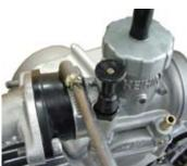
O Attach an air filter, which please fix by tightening a band.
