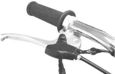
2 . Apply grease to the sliding surface on the throttle, and install the throttle housing. Tighten the pan screws.
