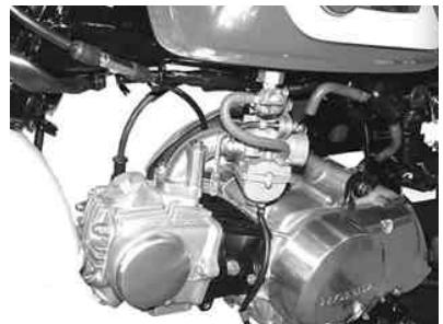
11 . Pull the choke lever to start the engine, and check for any intake gas leak. Gradually push the lever back and warm-up the engine till it starts running smoothly, and push back the choke lever to the end. Adjust the throttle stop screw in case the engine does not run idle after the warming up or runs idle at high speed.
