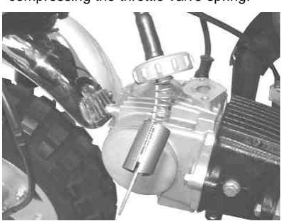
5 . Mount the throttle valve to the carburetor aligning the notch on the throttle valve with the throttle stop screw.
