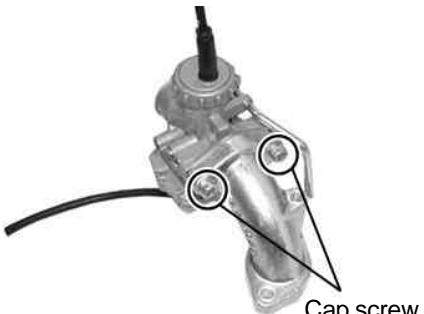
7 . Remove the cramp on the wire harness. Fix the wire harness, sliding it so that it will not interfere with the carburetor. Fix the gasket first and then the inlet pipe to the cylinder head. Tighten the 6x25 socket cap screws to the specified torque.
