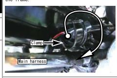
Connect throttle opening sensor connector, fuel injector connector, quick connector.
