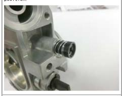
Attach the rubber seal and the removed parts to the big throttle body and tighten with specified torque.
