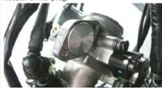
Attach socket cap screw (5x8) and plain washer (5mm) and tighten with specified torque.
