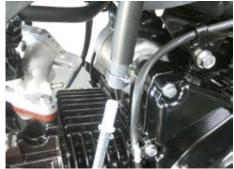
Remove the flange bolts, and remove the genuine throttle body.
