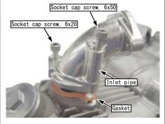
O Fasten the insulator to the inlet pipe with two socket cap screws.
