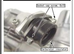
O Install the carburetor into the insulator and tighten it with the clamp band.
