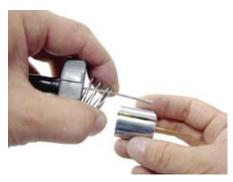
O Fix the throttle valve to the carburetor by aligning a notch on the throttle valve with the throttle stop screw.
