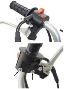
O Detach a stock throttle cable from the lower throttle housing.
