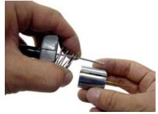
O Attach the throttle valve to the carburetor, aligning the notch with the throttle stop screw.
