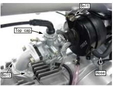
O Attach an earth cable to the frame with the bolt on the air cleaner stay.
