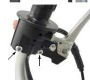
O Detach a stock throttle cable from the lower throttle housing.
