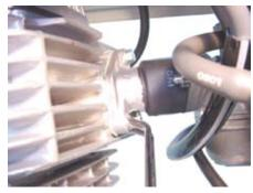
O Unfasten a pan head screw on the throttle housing from the motorcycle.
