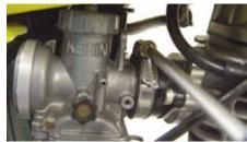
O Tighten the throttle-cable locking nut. % NOTE that fastening the locking nut too tight may break the housing.
