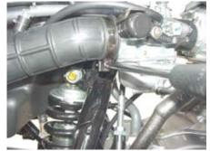
O Remove two case mounting bolts from the left side and one from the right side, all of which are fixing the stock air cleaner case.
