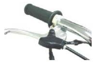
O Apply grease to the sliding surface on the throttle, and install the throttle housing.
