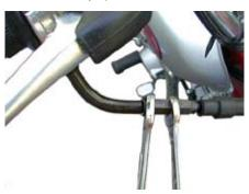
O Connect the fuel tube, open the fuel cock, and check each section for oil leaks.
