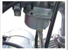
O Remove the fuel tube and throttle valve from the carburetor, and separate the throttle valve from the throttle cable.
