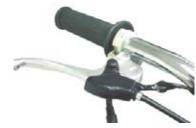
O After applying grease to the sliding surface of the throttle, install the throttle housing. Then tighten the pan screw
