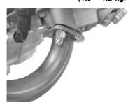
7 Next, tighten the flange bolt on the silencer stay to the specified torque.
