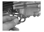
1 .Unfasten two nuts on the exhaust pipe flange. 1 . Remove the screws and bolts from the justnow-removed stock muffler, as shown by arrows in the below-mentioned photo, to
