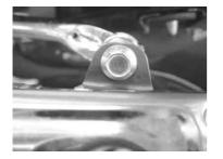
8 . Install the stock muffler guard. The stock plus screw will be reused. Place the supplied protector gaskets between silencer and muffler guard, and tighten the screw. As this screw is apt to come off from the vibrations of the vehicle, it is advisable to apply screw locking agent to it like a Lock tight 241, or the equivalent. Fix the front part of the muffler guard to the muffler by installing the protector band packing.
