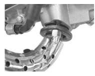
2 . Remove two hex bolts which are holding the muffler.
