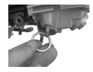
2 Fix a pivot nut onto the upper part of the right-side rear shock absorber. Torque : 35 N • m (3.5 kgf • m)
