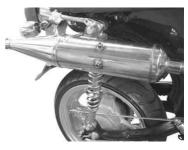
4 . After inserting the exhaust pipe into the joint on the silencer assembly, insert its flange into the engine.
