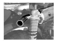
6 . Tighten the exhaust pipe flange nuts evenly to the specified torque with care not to let the silencer and the exhaust pipe get out of the adjusted places.
