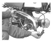
7 . Remove the old exhaust pipe gasket remaining in the exhaust port.
