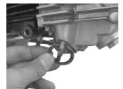
Reinstall the removed air cleaner in the order opposite to its removal.
