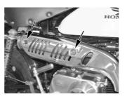
9 . Check for intereference among the genuine muffler guard, the muffler, and the frame. If need be, loosen the screws and nuts on each section to adjust the positions to the extent that the adjusting does not place too much strain on the muffler. Then fix them.
