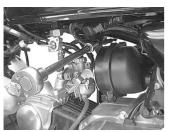
2 . Loosen the band which is clamping the carburetor and the air cleaner, and remove the air cleaner.
