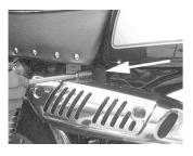
6 . After removing two collars on the exhaust flange, remove the muffler from the body by pulling it outward.
