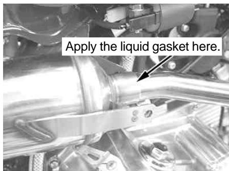
Apply the liquid gasket here.
