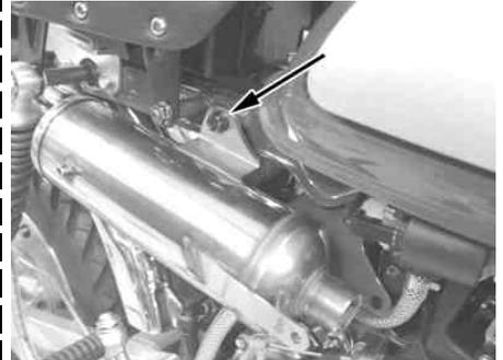
3. After inserting the exhaust pipe into the joint on the silencer assembly, insert its flange into the engine.
