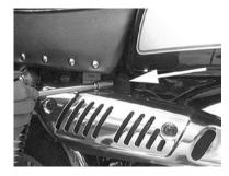
O After removing two collars on the exhaust flange, remove the exhaust system from the body by pulling it outward.
