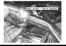
O Check the clearance between the exhaust pipe of canister and the rear fender, and then adjust the positions of the canister and the exhaust pipe so that they do not interfere with each other.
