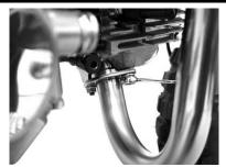
O Next, tighten the flange bolt on the canister bracket to the specified torque.
