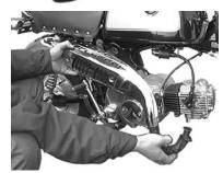
O Remove the old exhaust pipe gasket remaining in the exhaust port.
