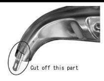
O If the exposing portion is cut off, it is advisable to give a touch-up to the cut surface with a heat-resistant paint to prevent the surface from rusting. ■ Mounting procedure ※ Please refer to the Genuine Service Manual for detailed mounting methods and specified torques that are not specifically described.
