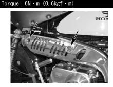
O Check for interference among the genuine exhaust system guard, the exhaust system, and the frame. If need be, loosen the screws and nuts on each section to adjust the positions to the extent that the adjusting does not place too much strain on the exhaust system. Then fix them.
