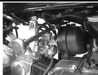
O Loosen the band which is clamping the carburetor and the air cleaner, and remove the air cleaner.
