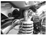
O Tighten the exhaust pipe flange nuts evenly to the specified torque with care not to let the canister and the exhaust pipe get out of the adjusted places.
