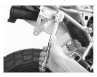
4 . Fit the silencer assembly into the exhaust pipe COMP.
