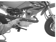
6 . Detach a used exhaust gasket in the exhaust port.
