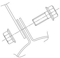
6 . First, adjust the positions of silencer and exhaust pipe. Then, being careful not to let these parts get out of place, tighten up the flange nut on the cylinder- head exhaust port equally to the specified torque.
