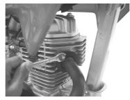
4 . Remove two flange bolts securing the muffler. Keep these flange bolts, which you will be re-using. And in case they are severely damaged, replace them with new ones.
