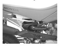
3 . Remove two nuts on the exhaust pipe.
