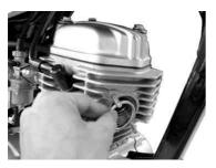
2 . Fit the exhaust pipe COMP. into the cylinder exhaust side, and tighten it loosely for now with a genuine nut.
