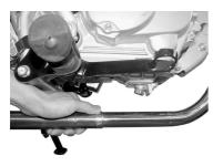
5 . Attach the band rubber to the inside of the clamp band, and fit the clamp band to the silencer. And secure it to the silencer stay for now with an 8x20 flange bolt and M8 flange
