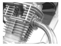
Secure the silencer stay to the genuine muffler stay on the bike with a genuine muffler bolt.
