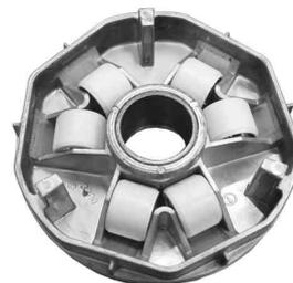
Be careful that no oil or grease will stain the movable drive face or spacer. Be sure to degrease the face or spacer whenever stained with oil or grease.
