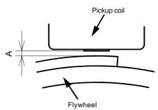
Please check the width of the opening A by putting a 1mm-wide wire through the opening A.
