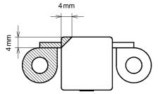
Chip away the shaded area with a grinder. Be careful not to chip the area too much, particularly the area in and around the portion where the lead wire is welded. Otherwise, the terminal will get exposed.
