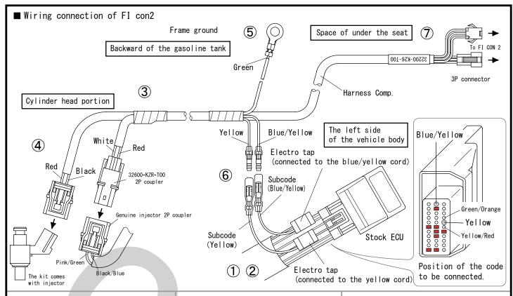
In order of the number in figure, do the work while checking the annotation.
