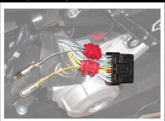
② Please put the electro tap part in the stock harness cover as much as possible and restored to securely connect the connector to the genuine ECU.
