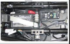
® Connect 3P connectors of FI CON2 with 3P connectors of harness Comp.
