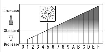
FI CON2 to match the vehicle individual differences and preferences, can be adjusted the correction value of the selected MAP by changing the rotary switch. "5" is the standard value of our setting, and more the number is smaller, the amount of fuel injection value will be decreased. More the number is bigger, the amount of fuel injection value will be increased. However, "0" is for the initial setting. If set to "0", engine will be stopped.
