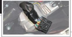
③ Put 2P connectors of the harness Comp. in a kit to the rear of the vehicle along with the main harness of the left side of the vehicle body surface to be able to connect to the stock injector connector.
