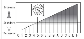
FI CON2 to match the vehicle individual differences and preferences, can be adjusted the correction value of the selected MAP by changing the rotary switch. "5" is the standard value of our setting, and more the number is smaller, the amount of fuel injection value will be decreased. More the number is bigger, the amount of fuel injection value will be increased. However, "0" is for the initial setting. If set to "0", engine will be stopped.
