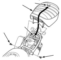
$\ensuremath{\mathsf{O}}$  Remove the battery bracket and battery, and remove the engine control unit.
