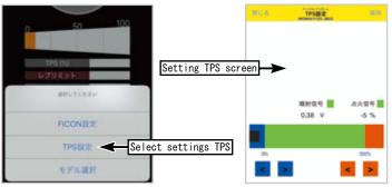
Try to fully close to fully open the throttle while waching the throttle position graph on the screen. The highlighted black moves from side to side in conjunction with opening and closing of the slot.
