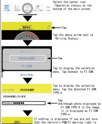
that the vehicle's PGM-FI warning light is flashing, turn off the main switch, fully open the throttle and turn on the main switch.
