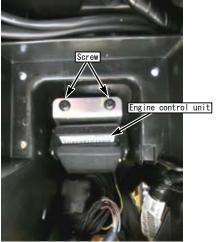
$\ensuremath{\mathsf{O}}$  Place and connect the FI CON TYPE-e between engine control unit and the main harness.
