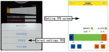
Try to fully close to fully open the throttle while waching the throttle position graph on the screen. The highlighted black moves from side to side in conjunction with opening and closing of the slot. Adjust each value with the level adjustment switch as match at the 0% and 100% positions. Please press "Save" when you done. It will not be reflected unless saved.
