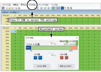
While looking at the throttle position graph on the screen, try to fully close to open the throttle. The gray highlight moves to the left and right in conjunction with opening and closing the slot. Adjust the level adjustment switch so that the values match at the 0% and 100% positions. Finally, be sure to press the "Save to FI CON" button. It will not be reflected unless saved.
