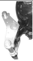
. Loosen the split clamp bolt on the steering stem, and adjust the right and left inner tubes evenly.
