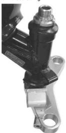
1 7 . Fit the front fork to the steering stem with the whirl stop on the axle holder on the right viewed in the direction of travel. And tighten an 8x20 steering-stem split clamp bolt loosely for the moment.
