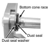
1 5 . Apply grease to the top cone race and bottom cone race, and attach the bearing to the steering stem and head pipe, and then the top cone race to the head pipe. In case the balls are not set in the bearing housing, then install 21 balls each to the bottom cone race and top cone race. Before applying grease, first wash the bearings with a solvent. Be careful not to let the dirt adhere to the bearings.
