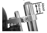
1 9 . Tighten the split clamp bolt on the steering stem to the specified torque.
