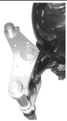
1 8 . Loosen the split clamp bolt on the steering stem, and adjust the right and left inner tubes to protrude in the same length. Protrude the inner tube about 30 mm so the caster angles become the same as the stock caster angles
