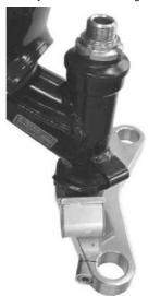
1 4 . Fit the front fork to the steering stem with the whirl stop on the axle holder on the right viewed in the direction of travel. And tighten an 8x20 steering-stem split clamp bolt loosely for the moment.
