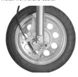
1 6 . Put a collar in between the front fender stay and bottom case, attach the 6x15 button head screw, and tighten it to the specified torque.
