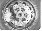
6 . Fasten the caliper to the caliper bracket with an 8x12 socket cap screw.
