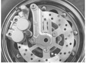
Align the concave portion of the caliper bracket with the convex portion of the front fork.
