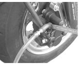
Release the brake lever slowly, and keep the lever in the fully released position for a few seconds.
