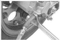
Connect the transparent bleeder hose to the bleeder valve on the rear caliper, and place a suitable cup at the other tip of the hose to receive brake fluid.
