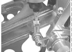
Turn the push rod on the master cylinder COMP, and adjust the location of the brake pedal. And tighten the 6mm hex nut (clockwise screw) to lock the pedal.
