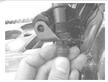
Install a rear stop lamp switch onto the stop switch stay.
