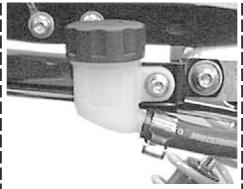
Add the brake fluid up to the upper level mark on the oil cup, and attach the diaphragm, diaphragm plate and cap.
