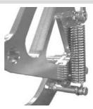
Fix a return spring to the following two: the 6x15 socket cap screw attached to the rear side of a brake holder, and the groove on the inside of a spring hook attached to the rear side of the brake pedal.
