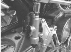
Route the brake hose so the brake hose COMP. will not stretch tight when the hose is compressed to a maximum. And tighten the banjo bolt to the specified torque.
