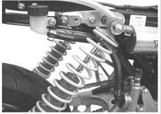
After deciding on how to route the oil hose, cut the oil hose. And attach it to the union on the oil cup and to the connector on the master cylinder COMP., and secure it with a hose clamp.
