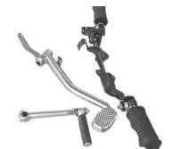
To remove stock brake pedals, unfasten a split pin holding the brake rod of stock brake pedals, and another split pin holding a brake return spring, stop switch spring and brake pedal.
