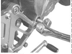
Install the kick starter arm. ▲ CAUTION : Be sure to follow the specified torque: Torque: 12N • m (1.2 kgf • m)
