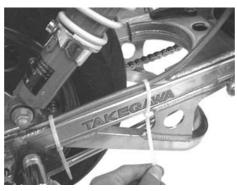
Secure the brake hose with a Tie Wrap so it does not interfere with other parts, and cut off the excess portion of the Tie Wrap with a nipper.
