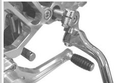
Set the positioning of the brake pedal so it does not interfere with the kick starter arm when you push down the kick starter arm to the end.
