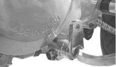
Install the supplied change arm to face upwards and tighten it.
