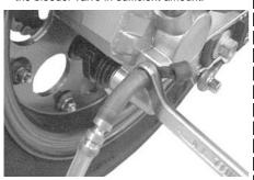
Do the work, adding new brake fluid, but paying heed to the amounts of brake fluid in the oil cup.
