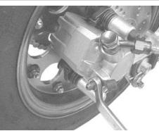
If you find that no more air is mixed, tighten the bleeder valve to the specified torque.
