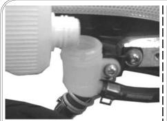
Detach the cap, diaphragm plate and diaphragm on the oil cup, and add the brake fluid up to the upper level mark on the oil cup.
