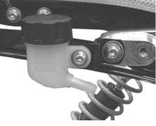
On the motorcycle equipped with our Rear Cowl Kit, install the reservoir tank stay to the tap on the seat stay with a 6mm plain washer and 6x20 button head screw.
