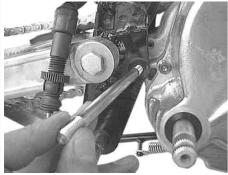
Replace the 8x98 mounting bolt in the lower part of the engine mount with a supplied
