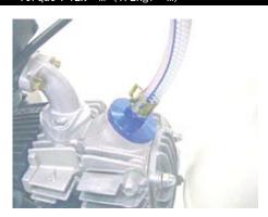
O Connect the hose of the crankcase breather, and fix it with a  $\phi$  9.5 hose clamp.
