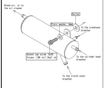
O Install the oil-catch tank onto a stock muffler-mounting spot. O Detach a hole cap from the clutch cover.
