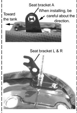
Just in the same way as a standard seat is installed, put the seat bracket in the space between two washers inside the rear shock absorber, and install a seat bracket A with a standard bolt and nut, and tighten them to the specified torque.
