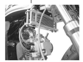
In the case of use with stock steering stem, since the steering angle is large, the oil cooler might be interfere with the steering lock.
