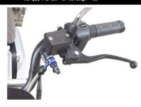
O As shown photo, pre-fix the brake hose fitting to the slim line banjo (straight) and route the hose note:not interfere any part of the exhaust pipe and steering wheel operation.
