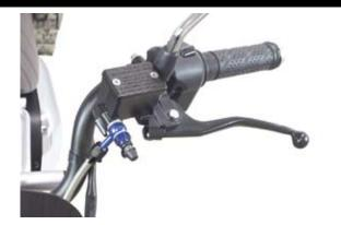
O As shown photo, pre-fix the brake hose fitting to the slim line banjo (straight) and route the hose note:not interfere any part of the exhaust pipe and steering wheel operation.
