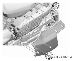
left pivot plate. Remove the M6x20 flange bolt and remove gear shift pedal.
