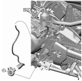
O Remove the four M8x20 flange bolts and 8.5x20 washers and remove the step.
